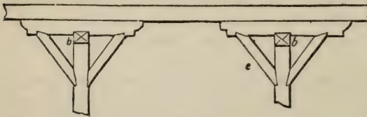
Fig. 101—Represents a horizontal beam c supported by vertical posts a, a, with corbel pieces d, d and inclined struts e, e to diminish the bearing.
